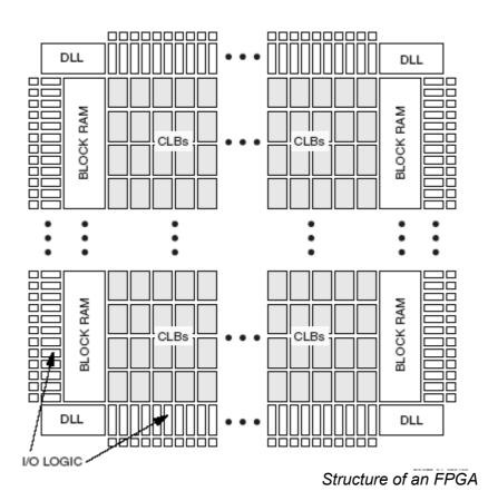
Beside the logic cells (CLBs) there can be found I/O-Blocks, internal memory (Block RAM), additional function blocks like multiplier or dlls (clock management)
